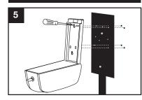
Using the hardware kit included, attach dispenser to mounting plate, and tighten firmly. (Hardware kit includes 4 screws and 4 lock nuts for attaching the dispenser.)
